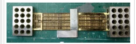
Here are two drilling jigs (and some machinists' blocks and a square) that I used to drill several holes in my On30 cars. So, I mentioned them in the CONSTRUCTION section of the write up and had them on hand during the evaluation for the team to review.
